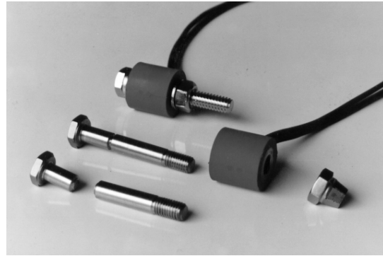
Fig. 2: Frangibolt™ separation system. The Frangibolt consists of an electric heater surrounding a hollow cylinder of TiNi and a specially-notched bolt. The TiNi actuator is prepared by compressing it 5 percent of its length, then securing it through the TiNi cylinder with a nut: a payload is secured for launch. To deploy the payload, electric power heats the TiNi actuator cylinder, it expands and elongates the notched bolt to fracture. A 1.5 cm diameter actuator delivers a force of 3 \times 10^5 newtons.
