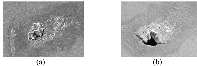
Figure 3: SEM shows two welded TiNi thin film after they were easily torn apart (a) a welded piece of TiNi thin film still attached but leaves a hole, as in (b), in the other film caused due to weakened film
