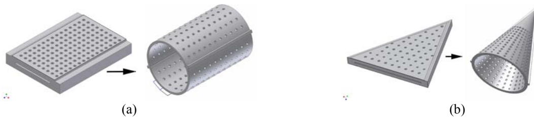
Figure 7: Computer-generated drawings to illustrate the transformation of planar multi-layer TiNi film into 3D structures (a) cylinder, and (b) cone after re-annealing with steel mandrel
